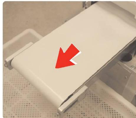
**If the conveyor belt moves in the opposite direction, press the “STOP/EMERGENCY” button 3 immediately thereby stopping the machine.**
