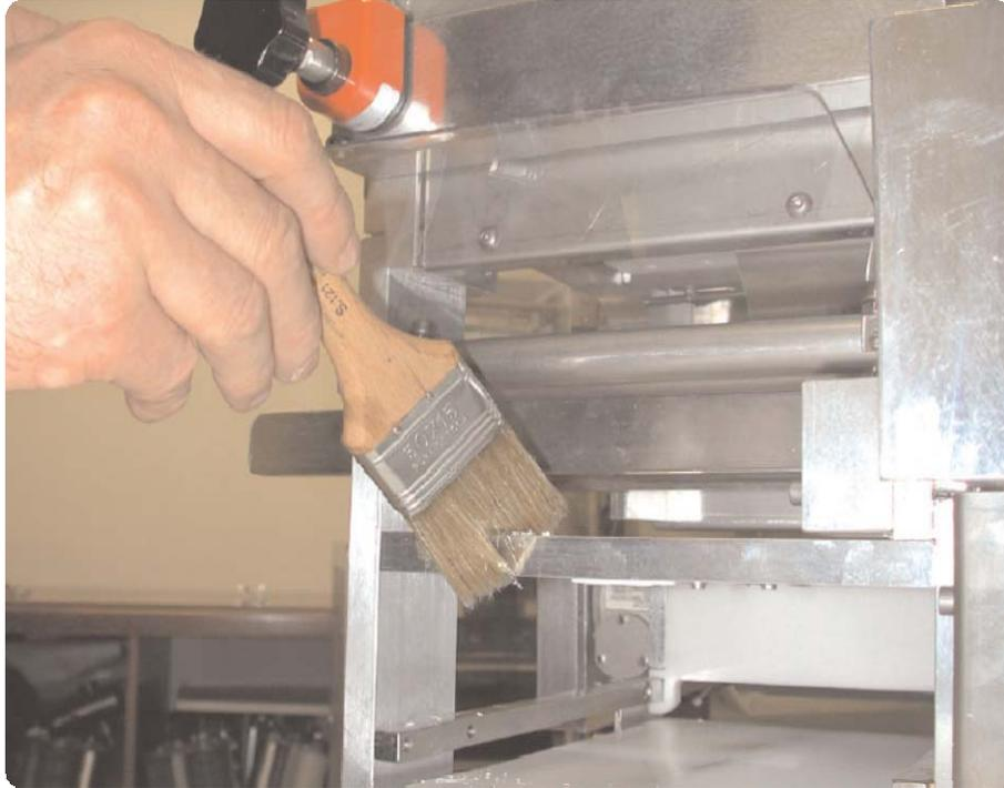
At the end of each working shift the machine must be cleaned. To undertake the cleaning, carry out the following operations:
