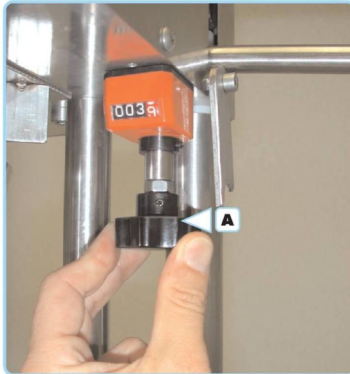
If the filling hollow is not centred, stop the machine when the grub screws on the cutting roller of the die are visible.
