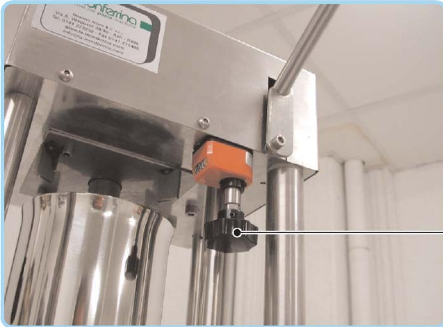
23 Hand wheel for regulation of quantity of filling.
